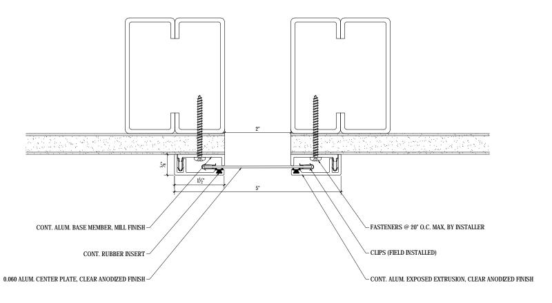
NOTE: 1 HOUR CONSTRUCTION INDICATED 2 LAYERS OF GYPSUM BOARD FOR 2 HOUR CONSTRUCTION
